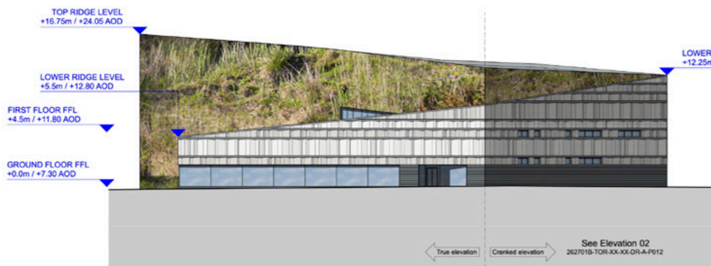
03 Elevation 03 (north-eastern) 1:200 @ A1 / 1:400 @ A3
